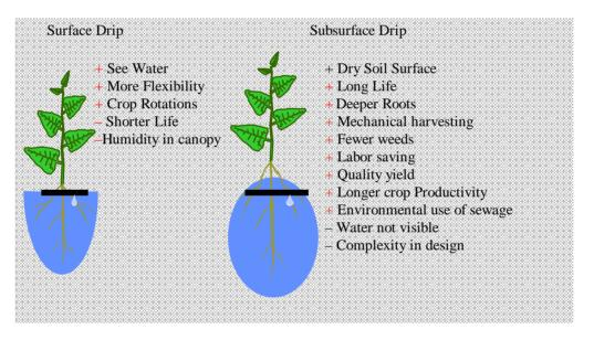
Technical advantages: Prevention of damage to irrigation equipment caused by machinery during cultivation and harvesting. It prevents equipments and land from damage caused by animals & birds. Movement of agricultural vehicles and machines minimize soil compaction along the rows. At the end of each season there is no need to lay-out, retrieve and re-connect the irrigation system. Irrigation of grazing land will be protected without causing obstructions (unlike sprinkling or flooding).
